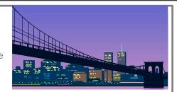
A suspension bridge is one where <u>cables</u> (or ropes or chains) are strung across the river (or whatever the obstacle happens to be) and the deck is suspended from these cables. Modern suspension bridges have two tall towers through which the cables are strung. Thus, the towers are supporting the majority of the roadway's weight.
